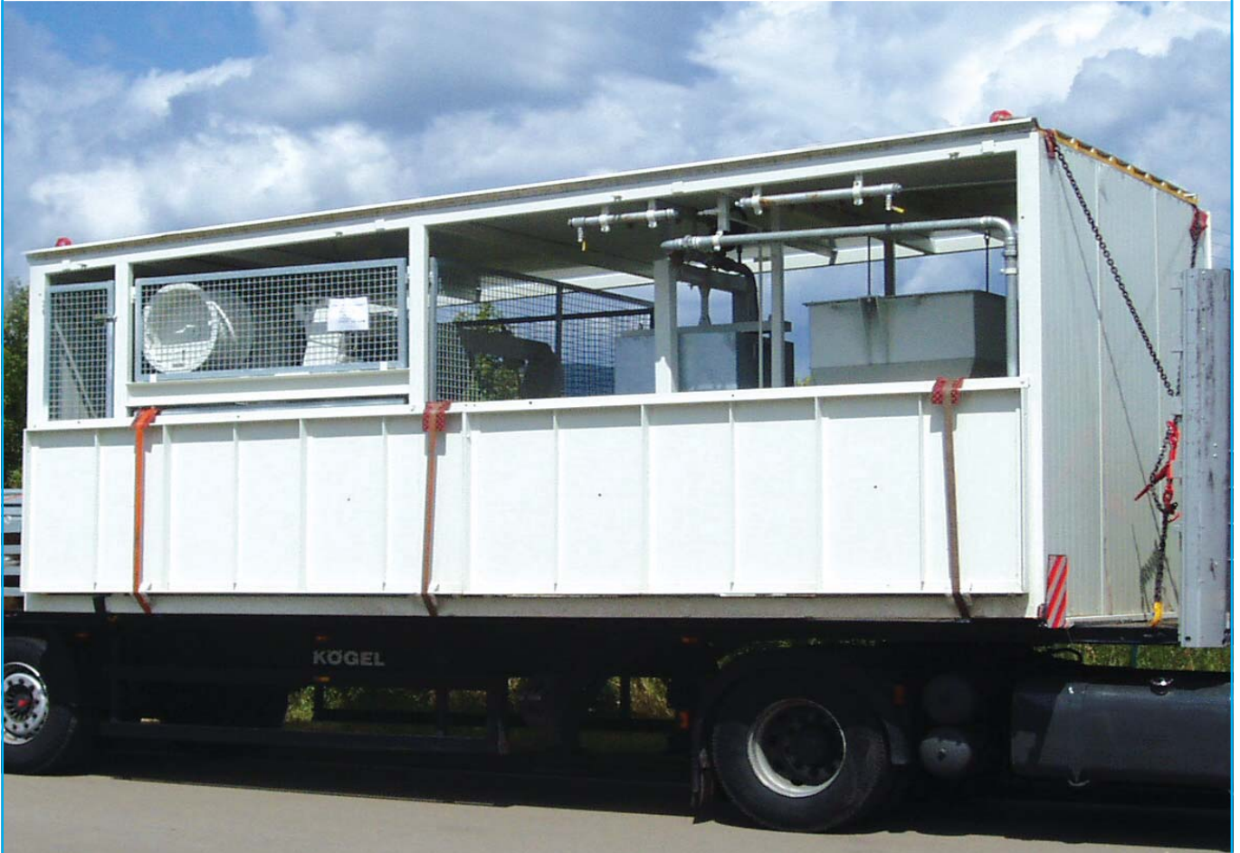
MIXOMAT THZ 3000 C - R Reihen-Siloanlage, Verladung des Waagen-Moduls • MIXOMAT THZ 3000 C - R aggregate in-line silo system, loading of a weighing module
